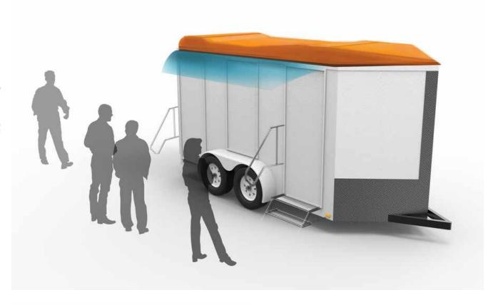
Each unit will cost \$59,560, apportioning 2 shower stalls with ample dressing space. Design of its interior allows the unit to be easily cleanable and maintainable: the walls and furniture will be constructed out of vividly colored stainless steel, and naturally anti-bacterial teak wood.
